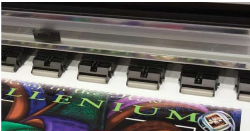
Fig. 1: The ValueJet's precision is largely due to the media handling, which features grips or hold-downs all across the printer.
