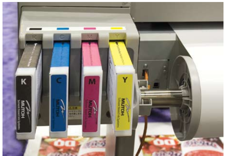
Fig. 4: The ValueJet snap-in, eco-friendly, solvent-based ink cartridges provide a scratch-resistant image. The printer uses Mutoh's new Eco-Ultra ink sets.
